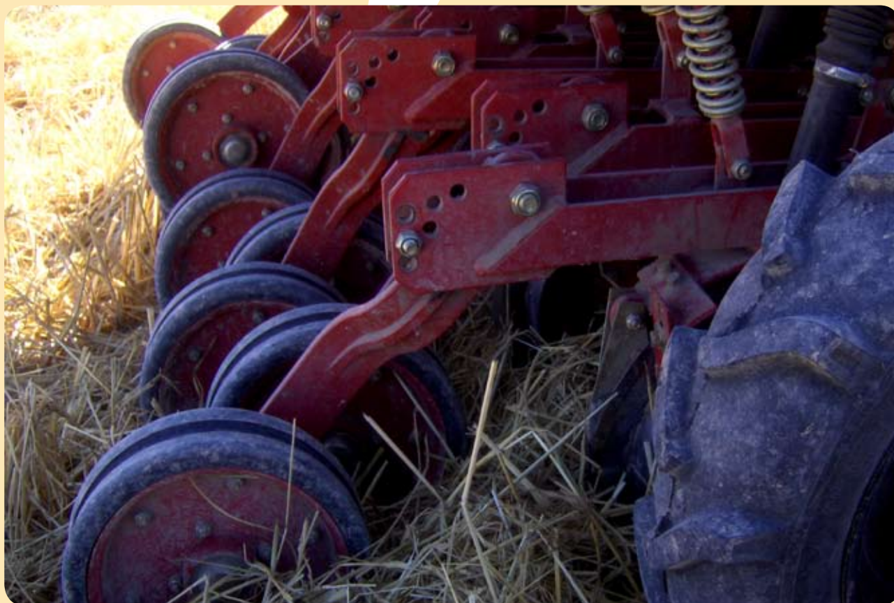
A working part of a sowing machine with a disc couler.
