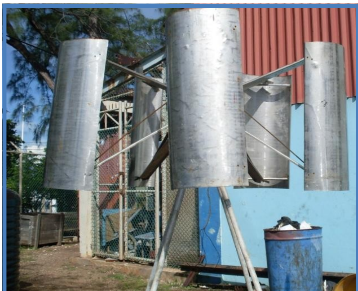
Wind turbine produced from recycled oil barrels
