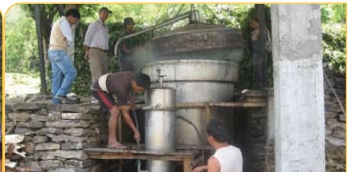
Extracting essential oil in steel lining distillation unit
