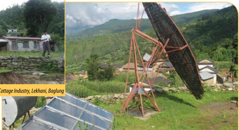
Parabolic solar cooker for Lokta boiling
