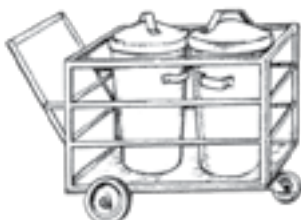
Waste vehicle that can be loaded with either containers or plastic bags
