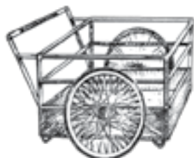
Waste vehicle with opaque floor and partly opaque sides
