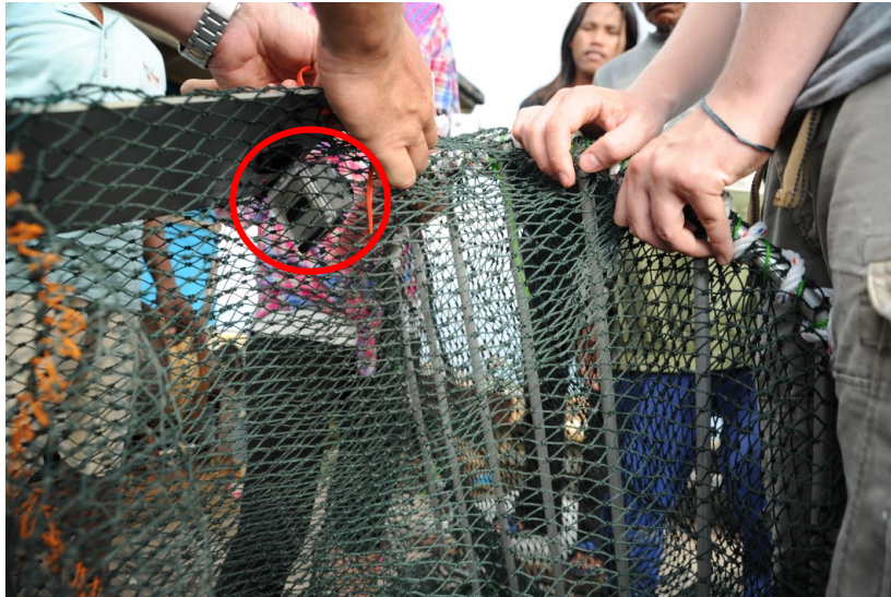
Figure 7. Video camera (circled in red) being attached to upper reach of the net in front of the TED grid. The camera was stabilised by a 6 x 10 sheet of PVC with holes drilled in the four corners, attached to the net with cable ties.
