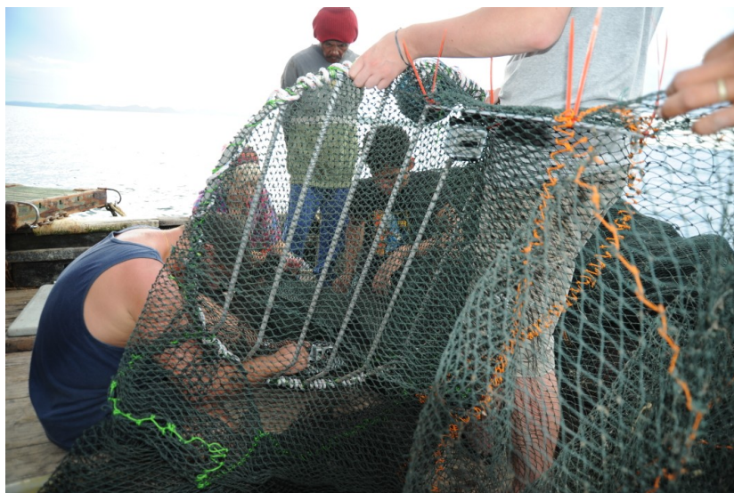
Figure 8. Video camera being attached to the lower reach of the net behind the TED grid (note upside down camera in front of the TED up top).
