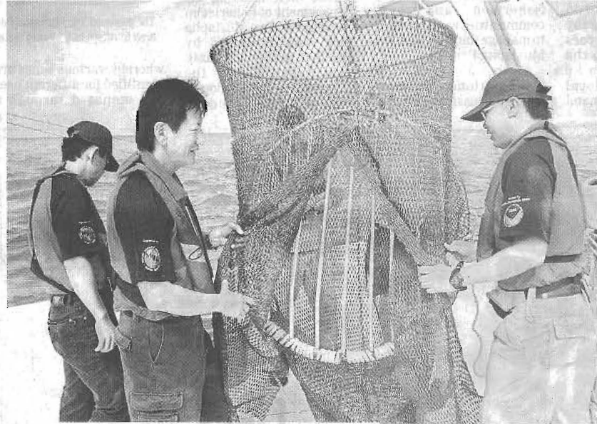
A trawl net equipped with TED being used in the pilot project.
