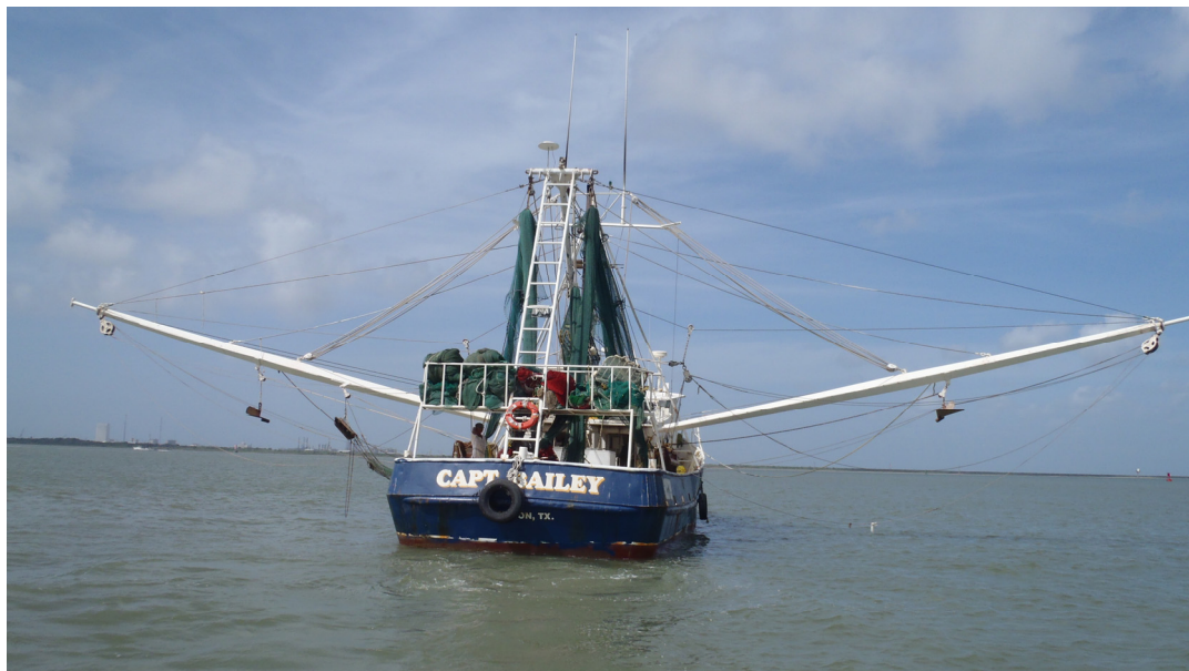
Figure 15. A twin trawl fishing boat with outriggers to spread two sets of nets and otter boards.
