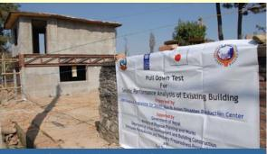
A retrofitted building ready for the pull down test
