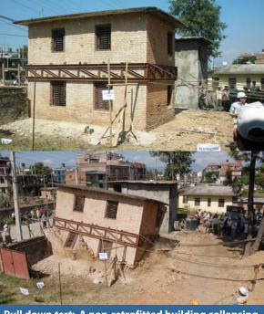
Pull down test: A non-retrofitted building collapsing
