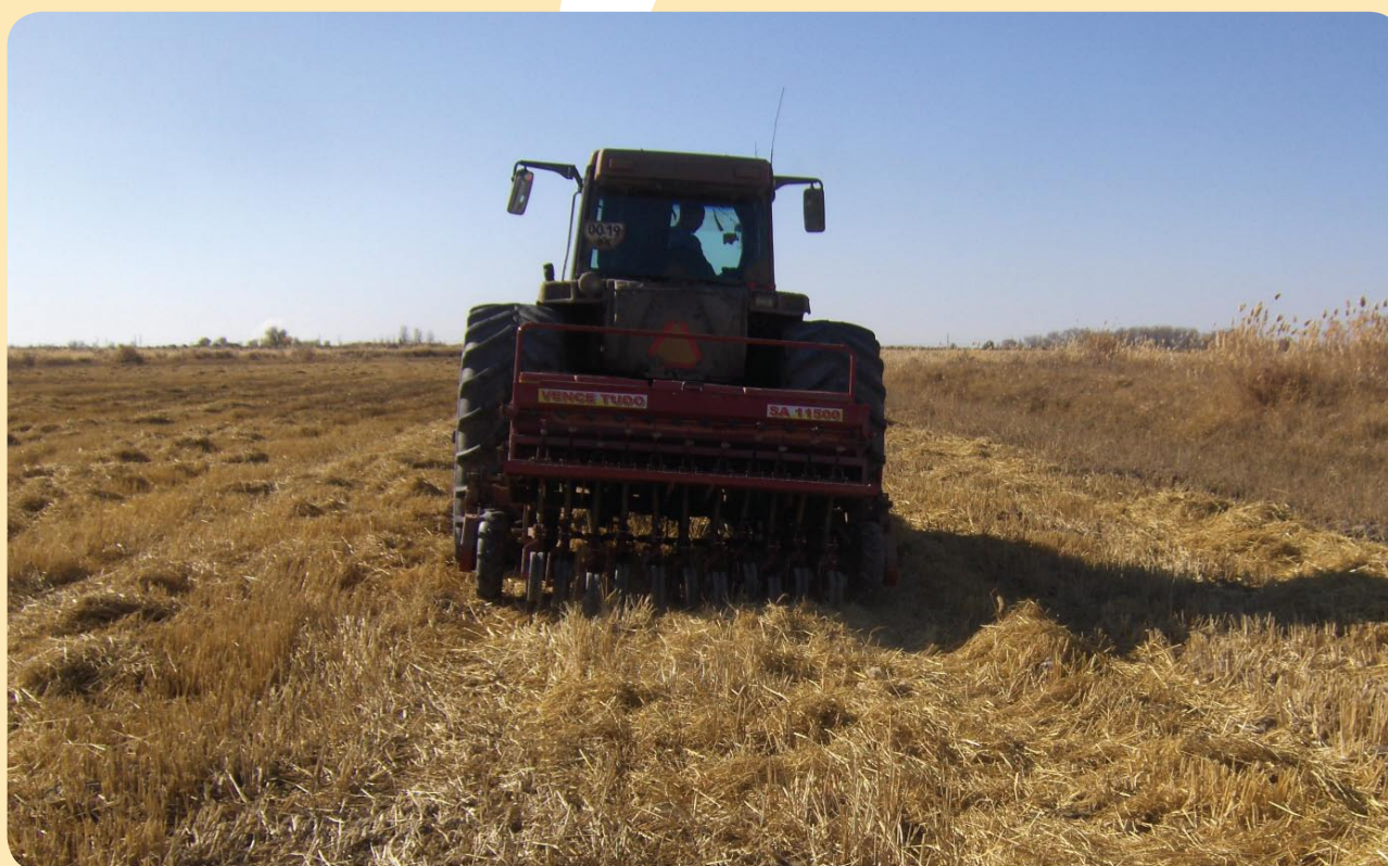
Photo 2. No-tillage experience in Karakalpakstan. A direct mulch seeding
