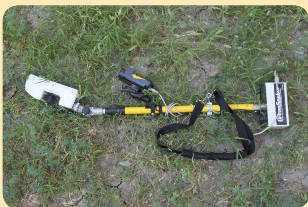
Photo 7. External view of the optical sensing device and its use on wheat, Urgench district, Khorezm province ( I. Kuryazov)
